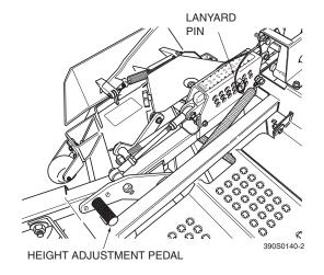
Figure 4-5. Adjusting Cutting Height
